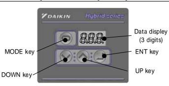
The operation panel is comprised of the 3-digit LED as shown in the left figure. There are four switch keys. Normally, the panel displays an actual pressure value
