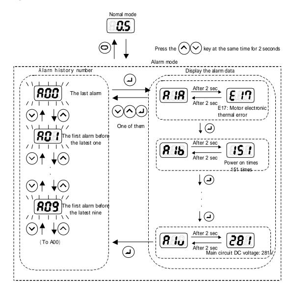
Press the  $\bigcirc$  key at the same time in normal mode. It will switch to alarm mode after about 2 seconds. Please press the  $\bigcirc$  or  $\bigcirc$  key to select the alarm history number. Display will flash if the alarm history number is under selection. A00 is the latest alarm, in the order of the A01  $\rightarrow$  A02  $\rightarrow$ , other old alarm histories
