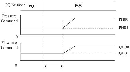
[P12: Solenoid valve response delay time]
