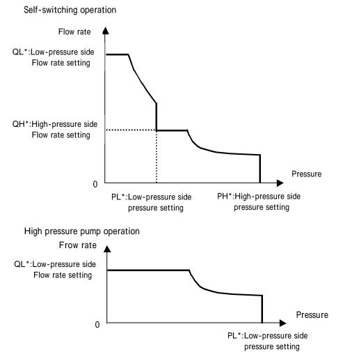
\* Please refer to "12.3.3 [P40: PL\_D] Settings when operating only at high pressure side (single) " for more information about how to set the high-pressure and low-capacity operation.
