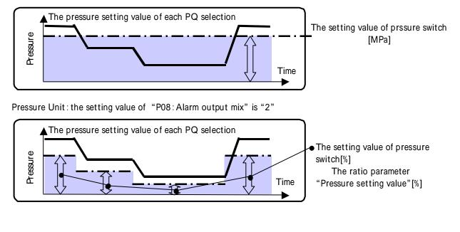
Pressure switch working example
