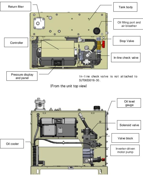
Solenoid valve is not attached to SUT06S3016-30 and SUT06S6007-30.
