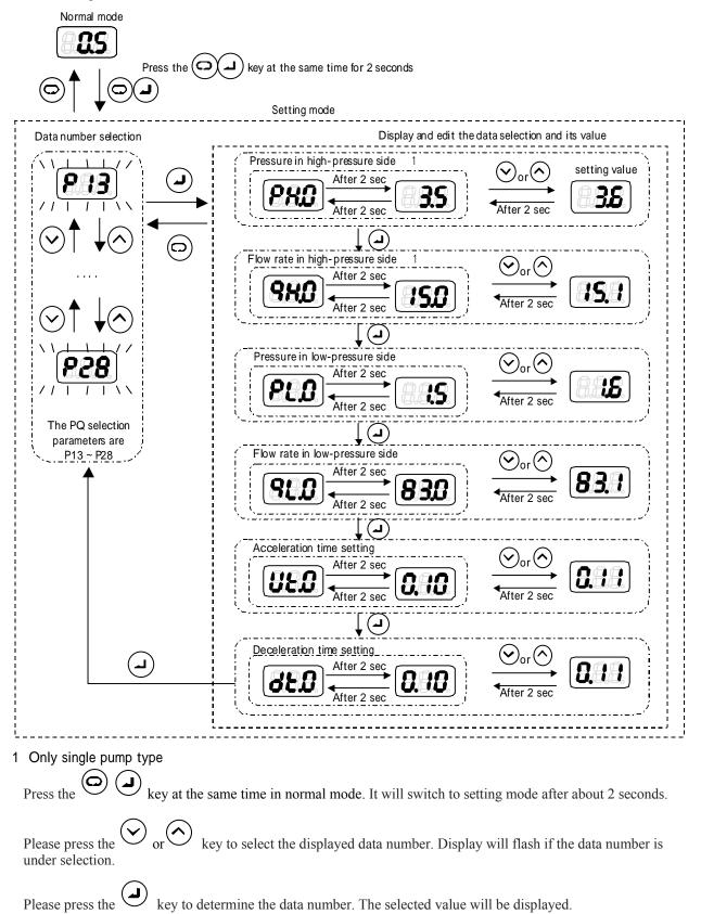
Each data symbol of PQ selection parameter and setting value are displayed alternately in about every two seconds.
