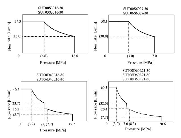
\*1 The above charts show the typical characteristics when the oil temperature is 40 °C. \*2 The above PQ characteristics show the usable range by actual flow rate.
