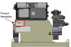
Front view of the Motor Pump type (SUT00)
